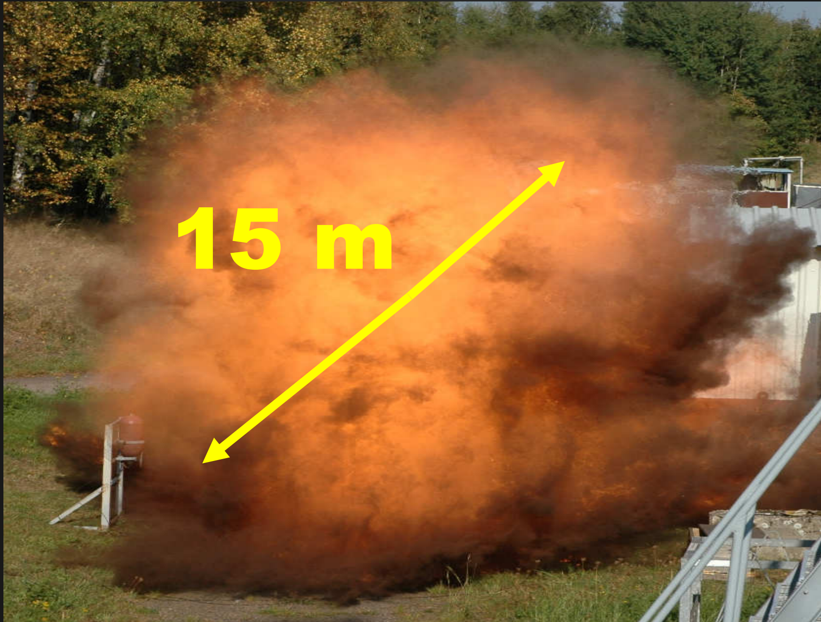
caused a fire ball with a diameter of 15 m.
