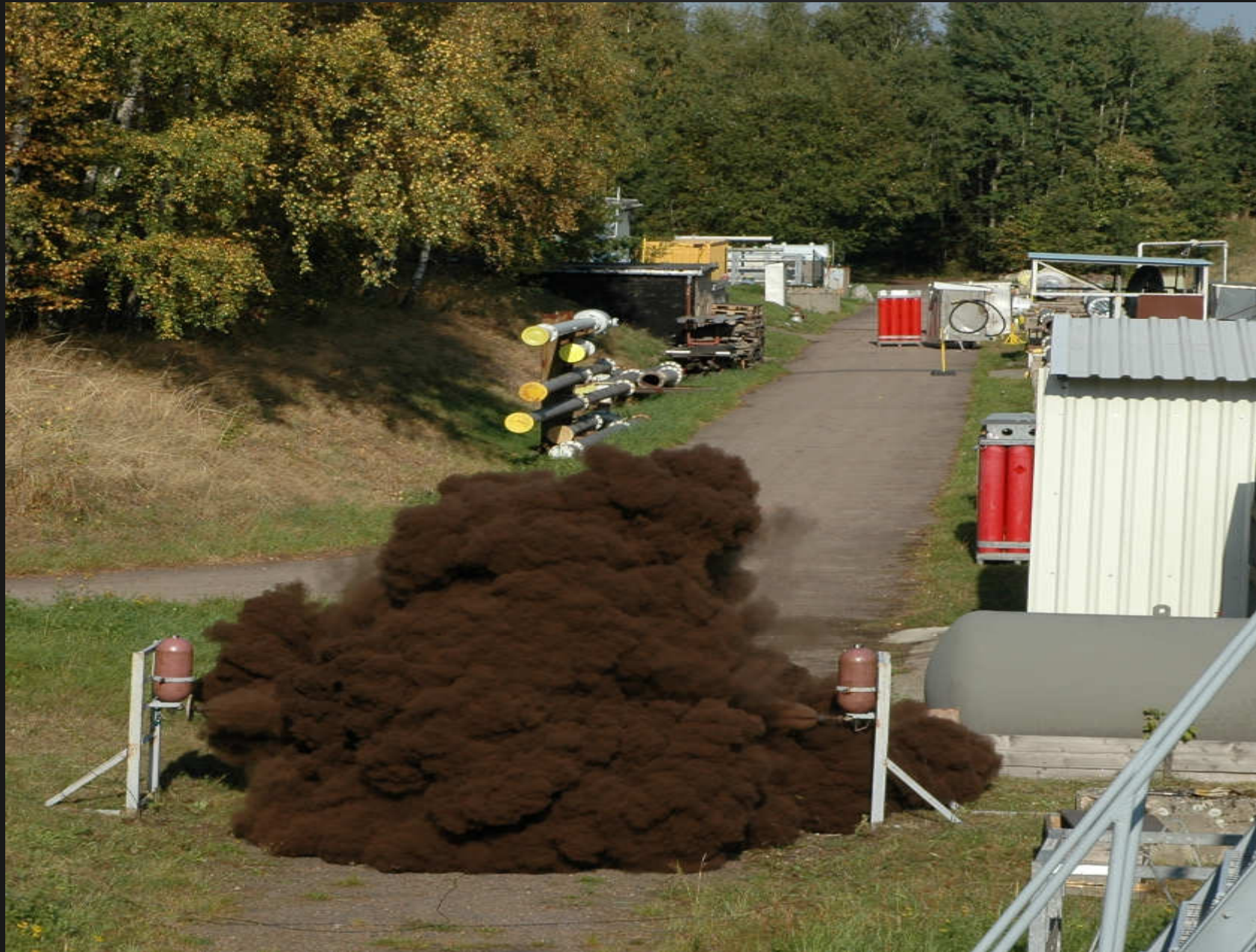
1,5 kg pulverized brown coal distributed in the air at the testing area of IBExU
