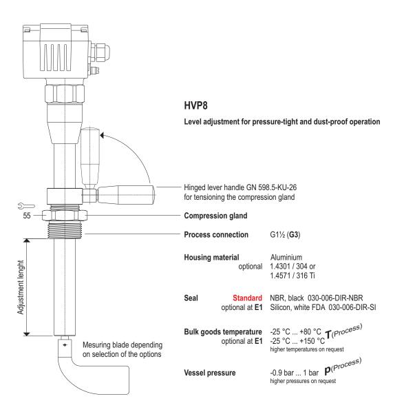
ATTENTION! At temperatures above +60 °C change the level adjustment only in cold condition or carry the appropriate safty gloves.
