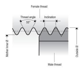
All couplings and pinch valves supplied by MOLLET are manufactured for cylindric connections with **not** metallically sealed threads.
